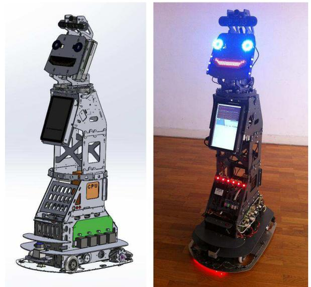
Figure 2. Mechanical drawing (left) and assembled platform (right).
